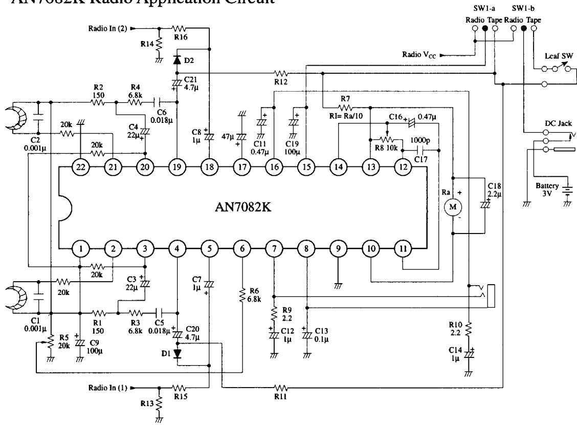
Note: Resistors R11/R12 and diodes D1/D2 are used to mute pre-amp during radio mode.
