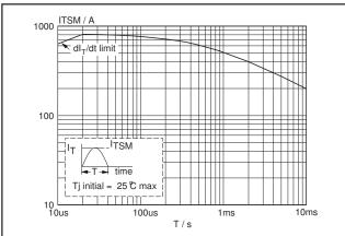
Fig.2. Maximum permissible non-repetitive peak on-state current  $I_{TSM}$ , versus pulse width  $t_p$ , for sinusoidal currents,  $t_n \le 10$ ms.
