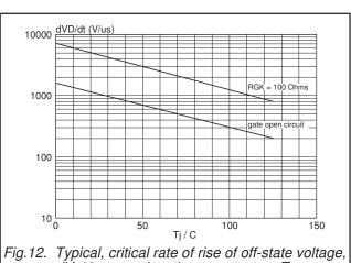
$d\dot{V}_D/dt$  versus junction temperature  $T_i$
