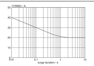
Fig.5. Maximum permissible repetitive rms on-state current  $I_{T(RMS)}$ , versus surge duration, for sinusoidal currents, f = 50 Hz;  $T_{mb} \le 103^{\circ}\text{C}$ .
