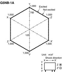
Quantity Tested: 5 units Test Method: Shock was applied 3 times in 6 directions along 3 axes and the level at which shock caused malfunction was measured. Rating: 100 m/s<sup>2</sup>
