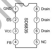
Note: it is recommended to connect pin 5 to pin Drain for better heat dissipation.
