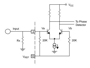
Figure 4. Desensitizing Input Stage
