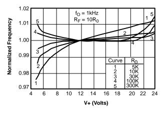
Figure 8. Typical f<sub>O</sub> vs. Power Supply Characteristics
