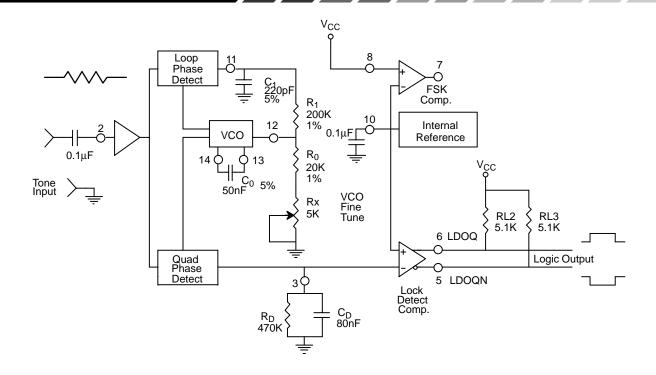
Figure 12. Circuit Connection for Tone Detection
