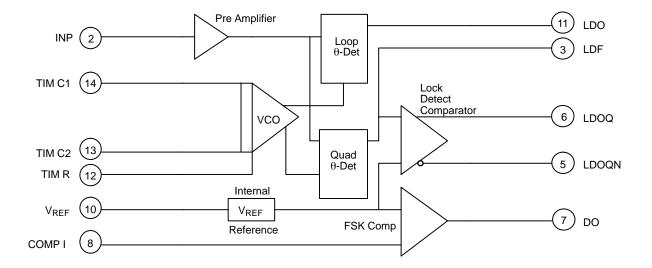
Figure 1. XR-2211 Block Diagram
