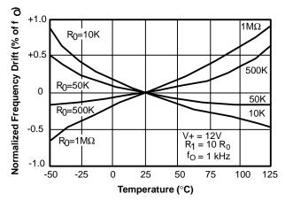
Figure 9. Typical Center Frequency Drift vs. Temperature
