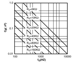
Figure 6. VCO Frequency vs. Timing Resistor
