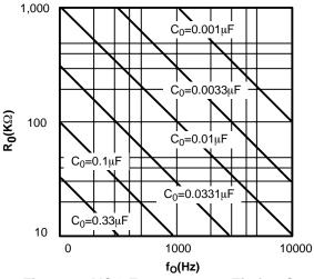
Figure 7. VCO Frequency vs. Timing Capacitor
