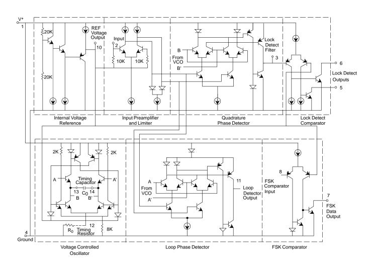
Figure 14. Equivalent Schematic Diagram
