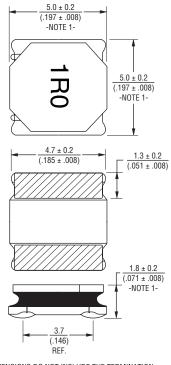
NOTE 1: DIMENSIONS DO NOT INCLUDE THE TERMINATION FOR MAXIMUM OVERALL DIMENSIONS WITH TERMINATION. ADD 0.1 MM (.004 IN.).
