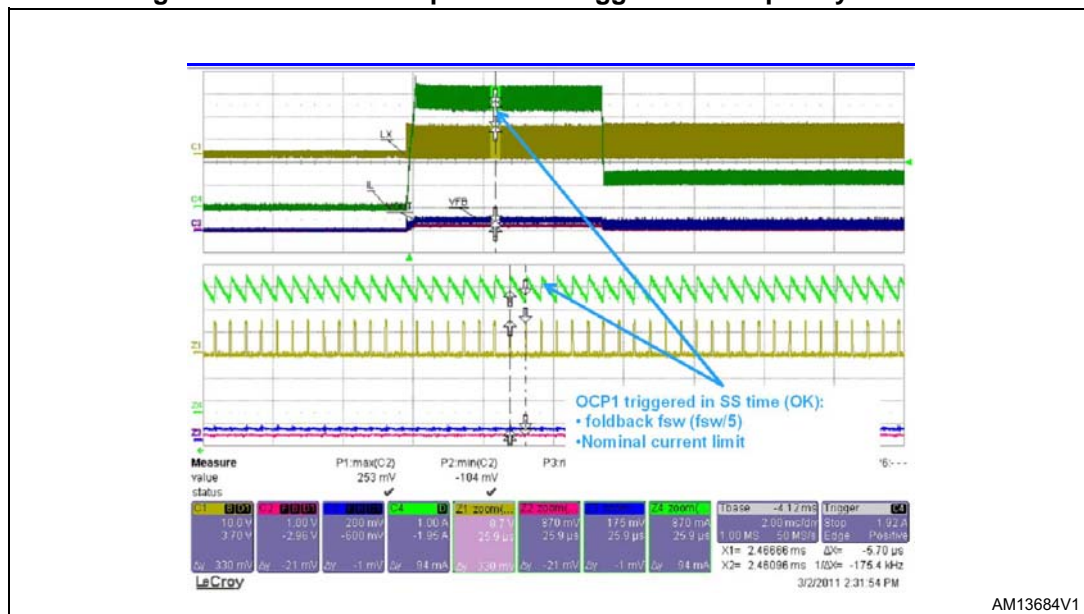
Figure 23. Over current protection triggers the frequency foldback
