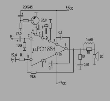
VCC MAX =  $\pm 30V$ VCC TYP =  $\pm 22V$ VCC RNG =  $\pm 17... \pm 23V$ Po = 18W RL = 8 Ohrn TDH = 0,1% ICCO TYP = 60mA ICCO MAX = 120mA IMAX = -RIN = -Gain = 40dB Noise = -RTHU-C = 3C/W Case SIP12H3 This datasheet has been downloaded from:
