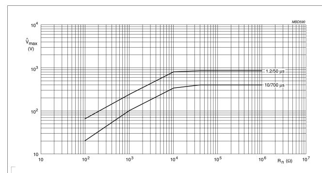
Maximum permissible peak pulse voltage without failing to open circuit' in accordance with DIN IEC 60040 (CO) 533 for type: RC0603
