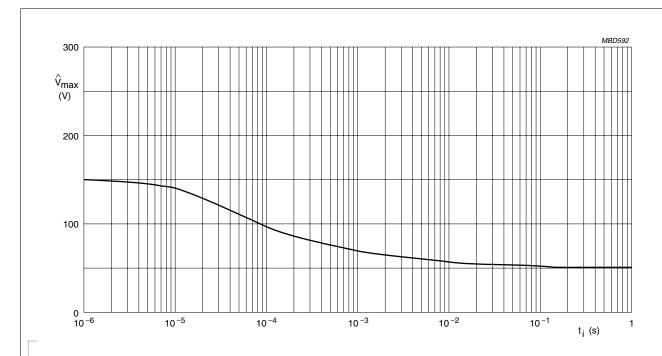
Fig. 9 Pulse on a regular basis for type: RC0603; maximum permissible peak pulse voltage as a function of pulse duration
