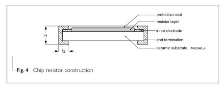
resistance value. Finally, the two external terminations (pure Tin) are added. See Fig. 4.
