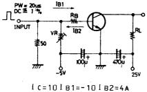
(For PNP, the polarity is reversed.) Unit (resistance : Ω, capacitance : F)
