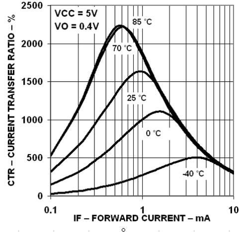
Figure 7: current transfer ratio vs. forward current
