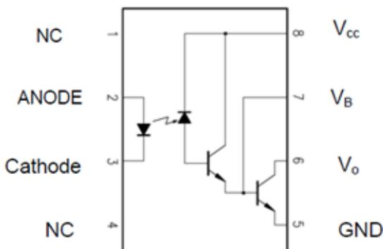
A 0.1μF bypass Capacitor must be connected between Pin8 and Pin5
