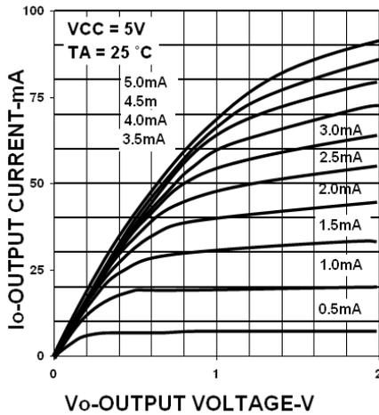
Figure 4: output current vs. input diode forward
