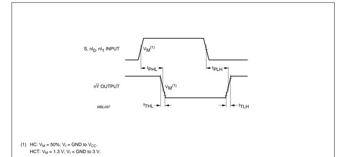
Fig.6 Waveforms showing input ( $nI_0$ ,  $nI_1$  and S) to output ( $n\overline{Y}$ ) propagation delays and output transition times.
