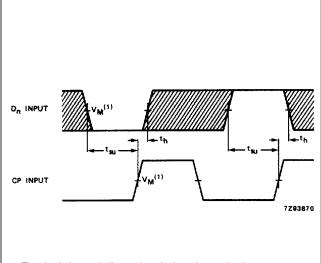
The shaded areas indicate when the input is permitted to change for predictable output performance.
