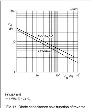
Fig.17 Diode capacitance as a function of reverse voltage, typical values.
