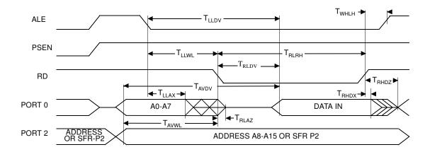
Figure 14-8. External Data Memory Read Cycle
