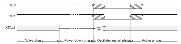
Exit from power-down by reset redefines all the SFRs, exit from power-down by external interrupt does no affect the SFRs.
