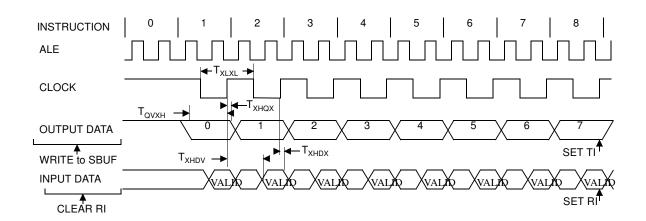
Figure 14-9. Shift Register Timing Waveforms
