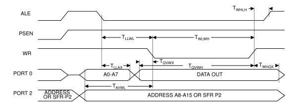
Figure 14-7. External Data Memory Write Cycle
