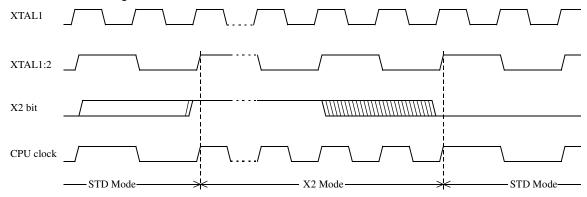
The X2 bit in the CKCON register (See Table 6-1.) allows to switch from 12 clock cycles per instruction to 6 clock cycles and vice versa. At reset, the standard speed is activated (STD mode). Setting this bit activates the X2 feature (X2 mode).
