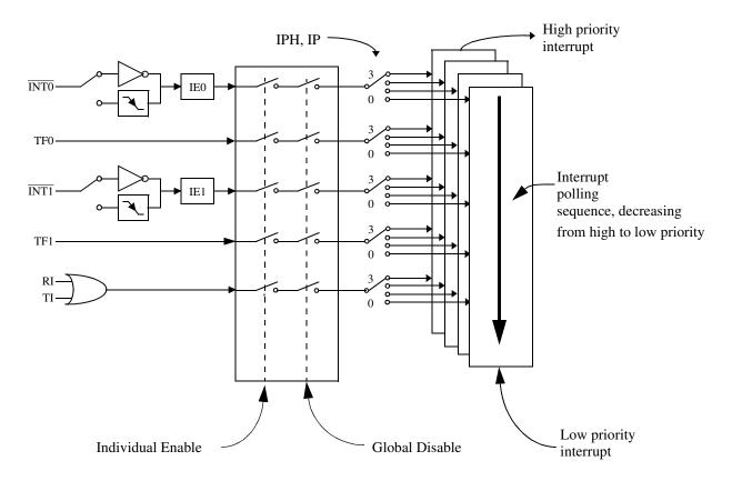
Each of the interrupt sources can be individually enabled or disabled by setting or clearing a bit in the Interrupt Enable register (See Table 10-2. Table 10-3.). This register also contains a global disable bit, which must be cleared to disable all interrupts at once.
