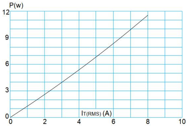
FIG.1: Maximum power dissipation versus RMS on-state current
