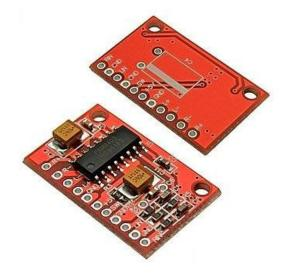
Ultra miniature digital amplifier board, the new high performance digital amplifier, input 5V to get  $[3 \times 2]$  6W power, ultra-thin board, Notebook external speakers, etc., as you imagine, the proposed power to take 5V or a single USB lithium powered.
