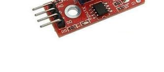
Two road red LED indicator: POWER and SENSOR. POWER: the power indicator will be lit up once powered—on. SENSOR: sensor indicator will be lit up once the sound detected by microphone reaches a certain point.
