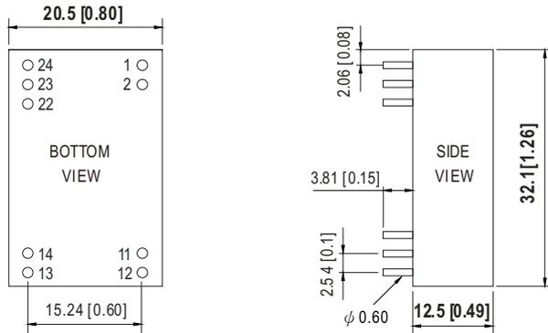
NOTE: Pin tolerance  $\pm 0.5$ mm
