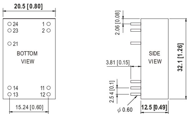
NOTE: Pin tolerance  $\pm 0.5$ mm
