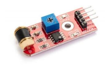
Main chip: LM393, vibration probe
