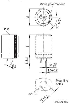
Snap-in terminals, length  $(6.3\pm1)$  mm. Also available in a shorter version with a length of (4.5-1) mm. PET insulation is marked with "PET" on the sleeve. Safety vent on the base.
