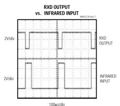
V<sub>CC</sub> = 3.3V, 2400bps AT 10cm DISTANCE, TERMIC BPV22NF, TRANSMIT POWER 200mW/sr
