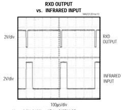
V<sub>CC</sub> = 3.3V, 2400bps AT 1m DISTANCE, TERMIC BPV22NF, TRANSMIT POWER 200mW/sr
