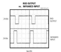
V<sub>CC</sub> = 3.3V, 115.2kbps AT 10cm DISTANCE, TERMIC BPV22NF, TRANSMIT POWER 200mW/sr
