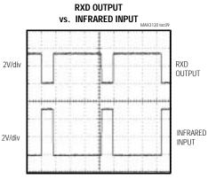
100µs/div V<sub>CC</sub> = 3.3V, 2400bps AT 1cm DISTANCE, TERMIC BPV22NF, TRANSMIT POWER 200mW/sr
