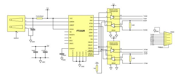
Figure 7.3 USB to RS422 Converter Configuration
