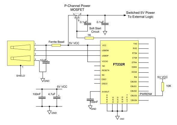
Figure 6.3 Bus Powered with Power Switching Configuration
