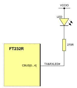
Figure 7.6 Single LED Configuration
