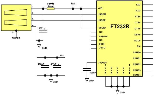
Figure 6.1 Bus Powered Configuration
