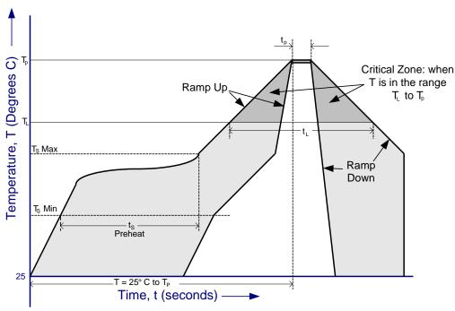
Figure 9.5 FT232R Solder Reflow Profile
