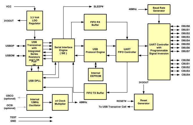
Figure 2.1 FT232R Block Diagram
