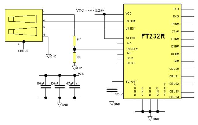
Figure 6.2 Self Powered Configuration
