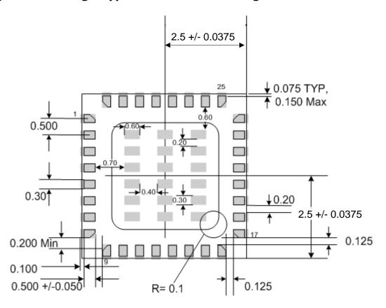
Figure 9.4 Typical Solder Paste Diagram for QFN-32 Package
