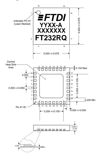
Note: The pin #1 ID is connected internally to the device's central heat sink area. It is recommended to ground the central heat sink area of the device.
