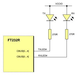
Figure 7.5 Dual LED Configuration
