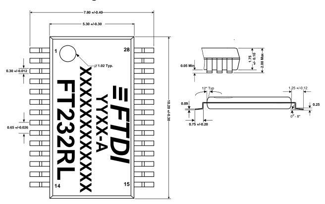
Figure 9.1 SSOP-28 Package Dimensions
