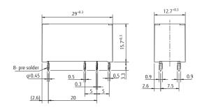
\*Dimensions of the terminals do not include thickness of pre-solder.
