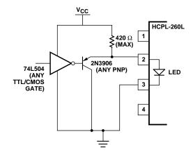
Figure 15. TTL interface circuit.
