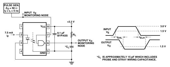
Figure 9. Test circuit for  $t_{\text{EHL}}$  and  $t_{\text{ELH}}$ .
