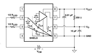
Figure 14. AC equivalent circuit.
