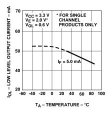
Figure 4. Typical low level output current vs. temperature.
