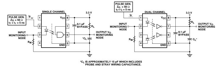
Figure 6. Test circuit for  $t_{\mbox{\scriptsize PHL}}$  and  $t_{\mbox{\scriptsize PLH}}.$
