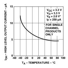
Figure 1. Typical high level output current vs. temperature.
