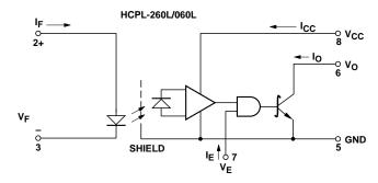
USE OF A 0.1 µF BYPASS CAPACITOR CONNECTED BETWEEN PINS 5 AND 8 IS RECOMMENDED (SEE NOTE 5).
