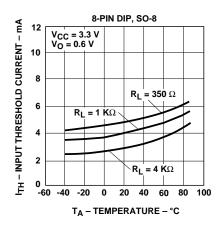
Figure 2. Typical input threshold current vs. temperature.
