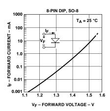
Figure 5. Typical input diode forward characteristic.
