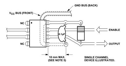
Figure 11. Recommended printed circuit board layout.
