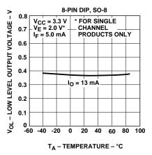
Figure 3. Typical low level output voltage vs. temperature.
