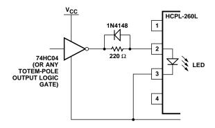
Figure 17. CMOS gate drive circuit.
