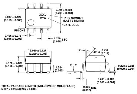
DIMENSIONS IN MILLIMETERS (INCHES). LEAD COPLANARITY = 0.10 mm (0.004 INCHES) MAX.
