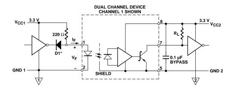
Figure 12. Recommended LVTTL interface circuit.
