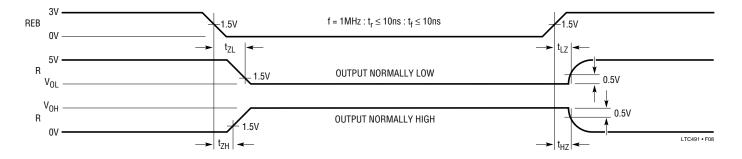
Figure 8. Receiver Enable and Disable Times
