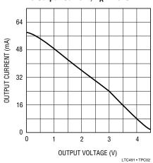
Driver Output Low Voltage vs Output Current, T<sub>A</sub> = 25°C
