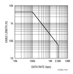
Figure 12. Cable Length vs Data Rate
