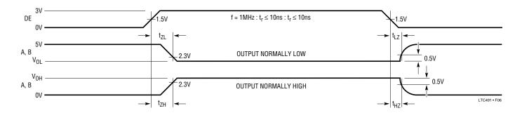
Figure 6. Driver Enable and Disable Times
