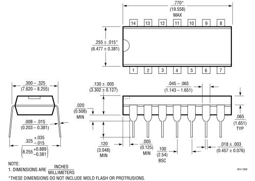
MOLD FLASH OR PROTRUSIONS SHALL NOT EXCEED .010 INCH (0.254mm)
