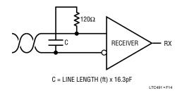
Figure 14. AC Coupled Termination
