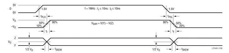
Figure 5. Driver Propagation Delays
