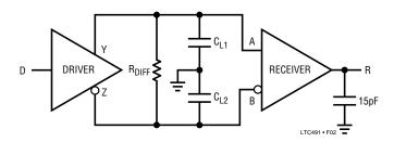
Figure 2. Driver/Receiver Timing Test Circuit
