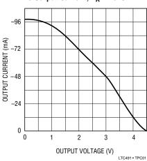
Driver Differential Output Voltage vs Output Current, T<sub>A</sub> = 25°C
