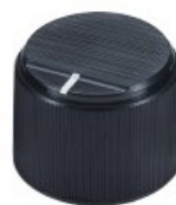
46110 Plastic knob with hair line polish on top with knurling and paint filled indicator line on top Material: ABS Diameter: 24.8 mm Height: 18.5 mm Shaft hole: \varnothing 6 mm, 18 Teeth
