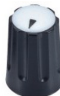
46116 Plastic knob with multi-color plastic cap, matte texture finish Material: ABS Diameter: 10.4 mm Height: 14.4 mm Shaft hole: \varnothing 6 mm, 18 Teeth
