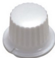
46124 Phenolic knob with ribs on O.D, glossy finish with one set screw Material: UREA, PHENOLIC Diameter: 23 mm Height: 14.6 mm
