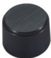
46111 Plastic knob with knurl and hair line polish on top Material: ABS Diameter: 30 mm Height: 20.5 mm Shaft hole: \varnothing 6 mm, 18 Teeth
