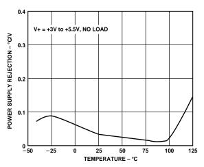
Figure 4. Power Supply Rejection vs. Temperature
