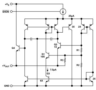
Figure 1. Temperature Sensor Simplified Equivalent Circuit
