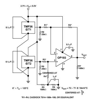
Figure 21b. Configuring Multiple Sensors for Differential Temperature Measurements
