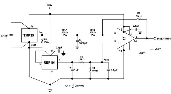
Figure 22. Pentium Over-Temperature Interrupt Generator
