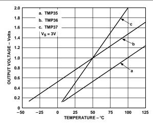
Figure 2. Output Voltage vs. Temperature
