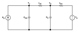
Figure 18. TMP3x Thermal Circuit Model
