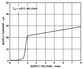
Figure 8. Supply Current vs. Supply Voltage
