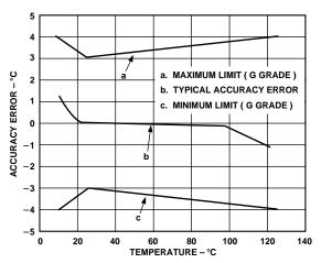
Figure 3. Accuracy Error vs. Temperature
