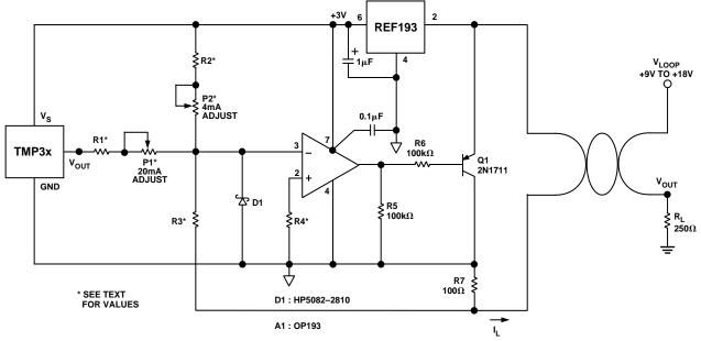
Figure 25. A Temperature to 4-to-20 mA Loop Transmitter
