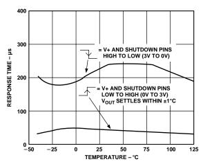
Figure 10.  $V_{OUT}$  Response Time for V+ Power-Up/Power-Down vs. Temperature
