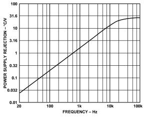
Figure 5. Power Supply Rejection vs. Frequency
