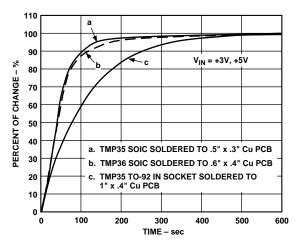
Figure 13. Thermal Response Time in Still Air
