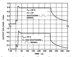
Figure 12.  $V_{OUT}$  Response Time to Shutdown and V+ Pins vs. Time
