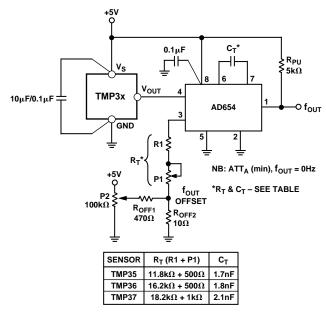
Figure 26. A Temperature to Frequency Converter
