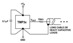
Figure 27. Driving Long Cables or Heavy Capacitive Loads
