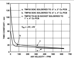
Figure 14. Thermal Response Time Constant in Forced Air
