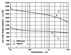
Figure 17. Voltage Noise Spectral Density vs. Frequency
