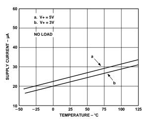
Figure 7. Supply Current vs. Temperature
