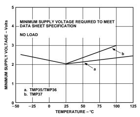
Figure 6. Minimum Supply Voltage vs. Temperature
