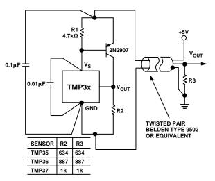
Figure 24. A Remote, Two-Wire Boosted Output Current Temperature Sensor
