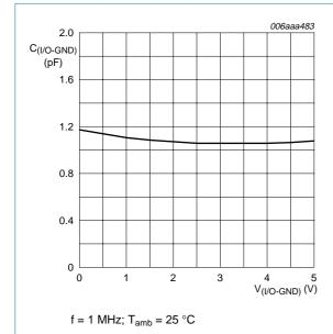
Fig 2. Input to ground capacitance as a function of input to ground voltage; typical values
