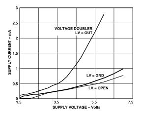
Figure 1. Power Supply Current vs. Voltage
