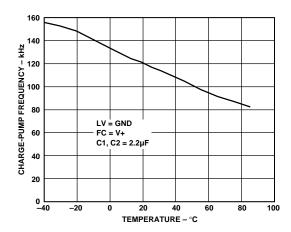
Figure 13. Charge-Pump Frequency vs. Temperature
