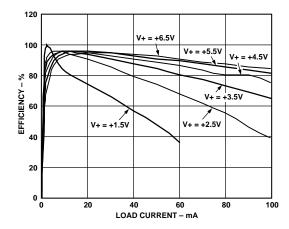
Figure 6. Power Efficiency vs. Load Current
