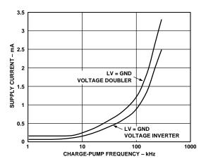
Figure 5. Power Supply Current vs. Charge-Pump Frequency
