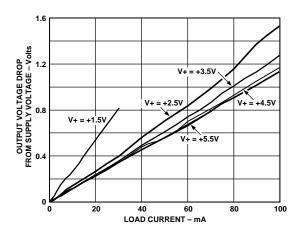
Figure 3. Output Voltage Drop vs. Load Current
