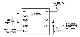
Figure 20. ADM8660 Voltage Inverter Configuration
