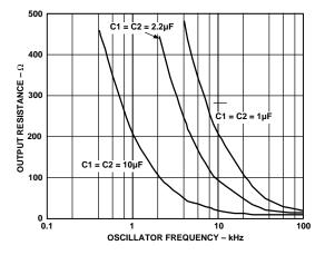
Figure 23. Output Impedance vs. Oscillator Frequency
