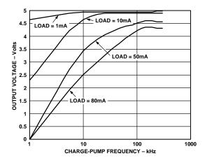
Figure 7. Output Voltage vs. Charge-Pump Frequency
