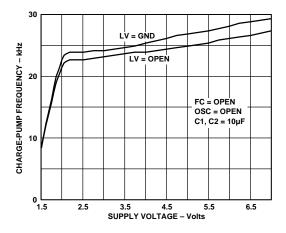
Figure 9. Charge-Pump Frequency vs. Supply Voltage
