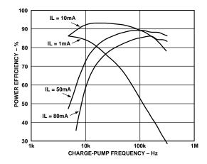
Figure 4. Efficiency vs. Charge-Pump Frequency
