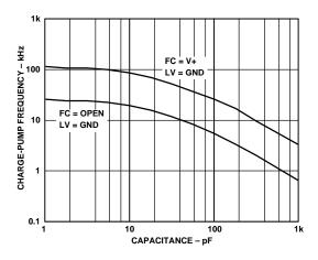
Figure 11. Charge-Pump Frequency vs. External Capacitance
