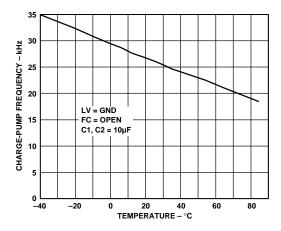
Figure 10. Charge-Pump Frequency vs. Temperature
