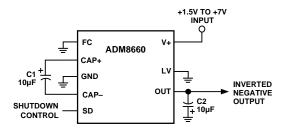
Voltage Inverter Configuration with Shutdown (ADM8660)
