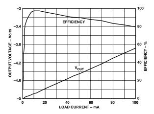
Figure 2. Output Voltage and Efficiency vs. Load Current
