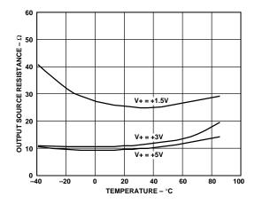
Figure 14. Output Resistance vs. Temperature
