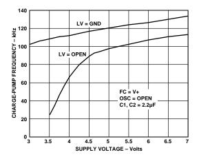
Figure 12. Charge-Pump Frequency vs. Supply Voltage
