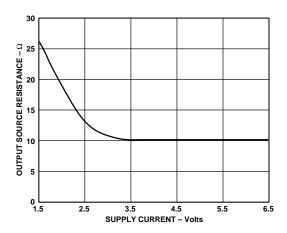
Figure 8. Output Source Resistance vs. Supply Voltage
