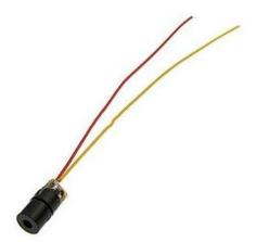
laser head Category: **o** 6.7 \* 10.5mm Size: Working life: more than 3000 hours Spot mode: point-like spot, continuous output Power:  $\leq 5 \mathrm{mW}$ Voltage: 3-6v (according to customer requirements) Current: <40mA -36 ℃ ~ + 65 ℃ Working temperature: Output Wavelength: 650 nm 10 meters at the spot for  $\mathbf{\phi}$  10mm  $\sim \mathbf{\phi}$  15mm Spot size: Band range: Visible Operation mode: Continuous Incentives: light pump Material: Plastic
