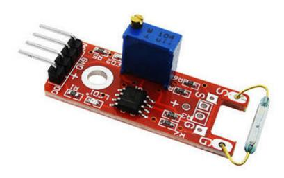
Use the magnetic module and the digital interface with 13 LED to build a simple circuit, making magnetic field indicating lights.
