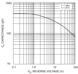
Fig. 4 Typical Junction Capacitance (per element)
