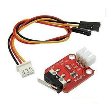
Simple circuit of Travel switch, collision module and integrated LED connecting to digital 13 interface to make collision flasher.
