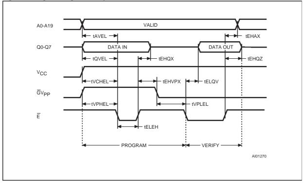
Figure 7. Programming and Verify Modes AC Waveforms
