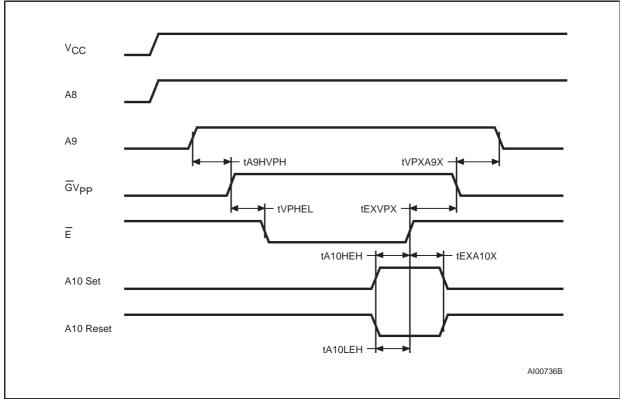
Note: A8 High level = 5V; A9 High level = 12V.
