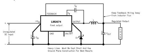
$C_{\text{IN}}$  - 22  $\mu\text{F},\,50\text{V}$  Tantalum, Sprague "199D Series"
