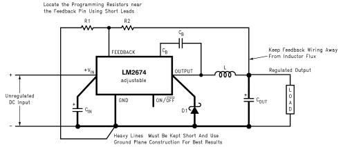
$C_{\text{IN}}$  - 22  $\mu\text{F}$ , 50V Tantalum, Sprague "199D Series"  $C_{OUT}$  - 47  $\mu F$ , 25V Tantalum, Sprague "595D Series" D1 - 3.3A, 50V Schottky Rectifier, IR 30WQ05F L1 - 68 µH Sumida #RCR110D-680L R1 - 1.5 kΩ, 1%  $C_B$  - 0.01  $\mu F$ , 50V Ceramic For a 5V output, select R2 to be 4.75 k $\Omega$ , 1%  $V_{OUT} = V_{REF} \left(1 + \frac{R_2}{R_1}\right)$
