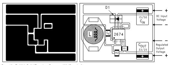
$C_{IN}$  - 15  $\mu$ F, 50V, Solid Tantalum Sprague, "594D series"  $C_{OUT}$  - 33  $\mu$ F, 25V, Solid Tantalum Sprague, "594D series"
