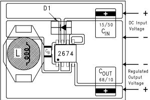
$C_{\text{IN}}$  - 15  $\mu\text{F}$ , 25V, Solid Tantalum Sprague, "594D series"
