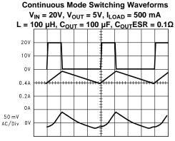
A: V<sub>SW</sub> Pin Voltage, 10 V/div.
