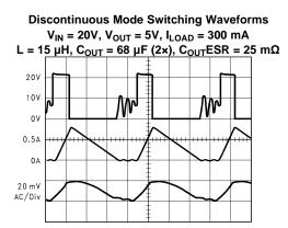
A: V<sub>SW</sub> Pin Voltage, 10 V/div.
